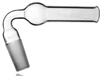
Guard Tube (to be filled with dry \text{CaCl}_2 )
