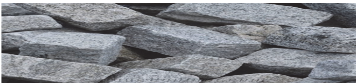
Fig. 1.2 Natural granite rocks dressed as per dimensional requirements called stones.
