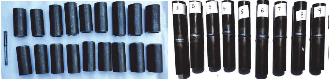
Figure 3: Samples of ASTM 106 Grade B Steel pipes, weldments
