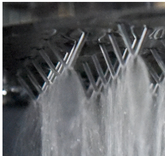
Figure 5: Impingement and fan formation of doublet oxidiser jets at 15% flow rate
