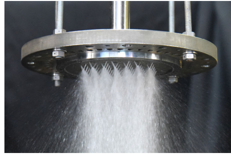
Figure 6: Impingement at 100% flow rate Figure 7: Impingement at 50% flow rate
