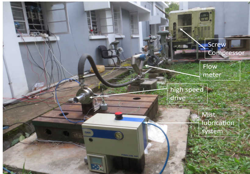
Figure 9: Facility established for testing of high speed drive
