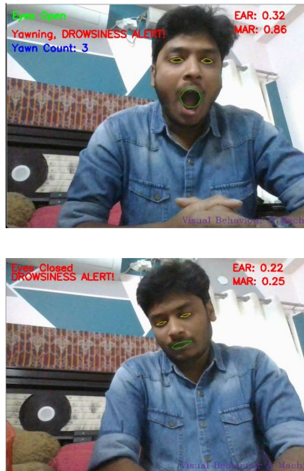
Figure 5: Drowsiness detected by the system due to (a) eye closing, (b) yawn, (c) head bending.
