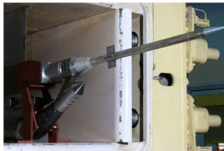
Figure 7: Basic Finner model in wind tunnel
