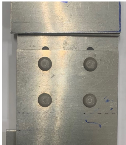
Figure 10: Rivet movement in slots after testing
