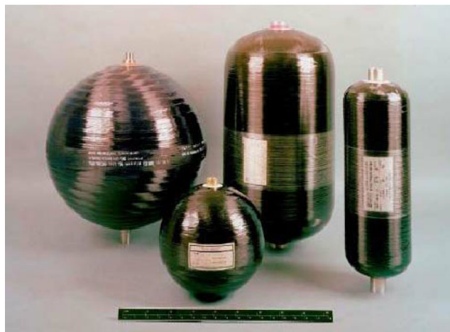
Figure 2: Composite overwrapped pressure vessels for gas storage [6]
