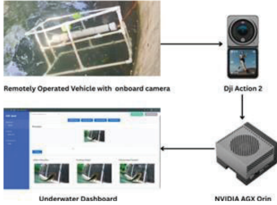
Fig. 1. Experimental setup with real-time UW-dash dashboard
