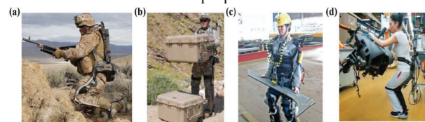
Figure 9 (a) HULC in combat operation, (b) HULC in payload lifting activity, (c) Industrial Exoskeleton for payload lifting, (d) Chairless chair exoskeleton supporting worker in industry
