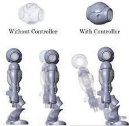
Fig. 11: Controller performance in terms of CoM position
