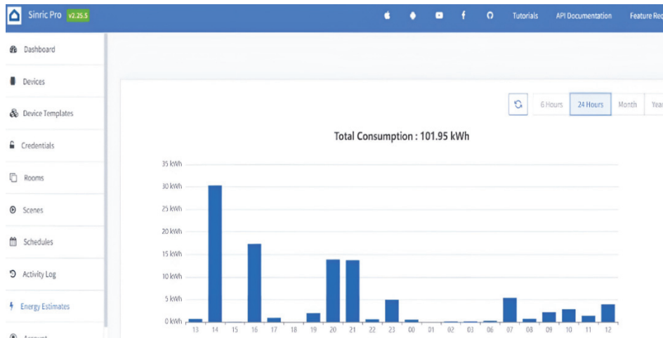
Fig. 3. Total Power Consumption for 24 Hours.
