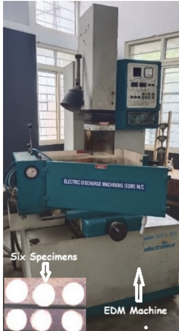
Figure 2: EDM 500 x 300 Electronica with machined component
