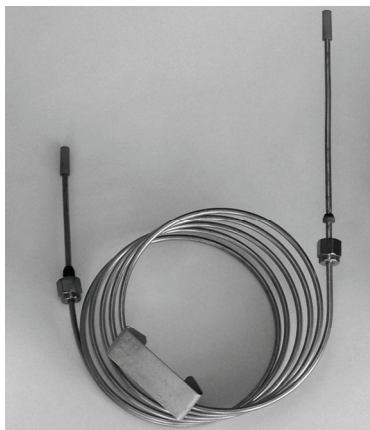
Fig. 1.6 A typically long GLC column (1 to 30 m) made into a coil
