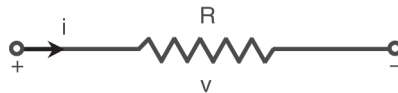
Fig. 1.16 Network model of a resistor and sign convention for voltage and current
